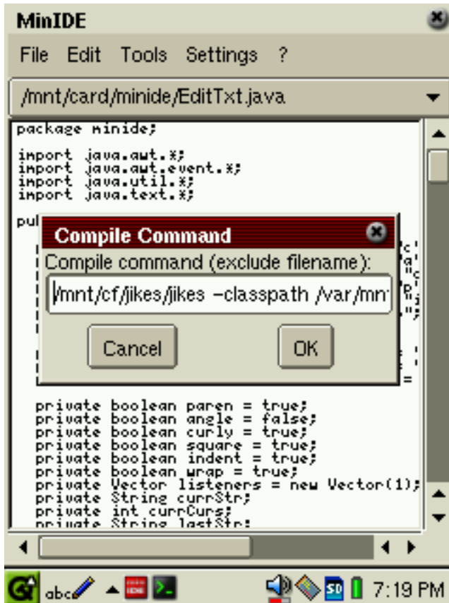
Figure 2: Use Settings -> Compile Command to enter the terminal command used to compile your files.
